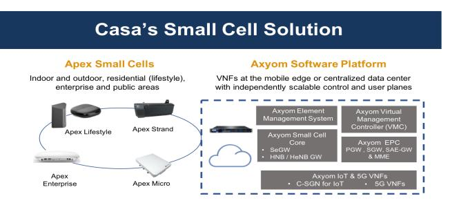
The Axyom Element Management System (AeMS) is an important part of Casa Systems' small cell solution, which includes Lifestyle and Enterprise small cells, Outdoor microcells, and the Apex Strand (a strand mount picocell) as well as virtualized high performance small cell gateways. The AeMS runs on Casa's Axyom Software Platform, which is a carrier-grade software architecture that provides the highest level of performance and control.
