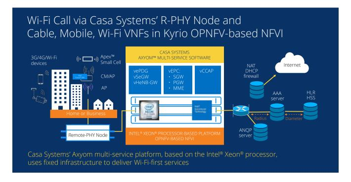
With regard to software, the PoC connects the R-PHY to a vCCAP core. Casa Systems' vCCAP and vEPC are installed in an OpenStack cloud running on a standard x86 server platform provided by Intel.
